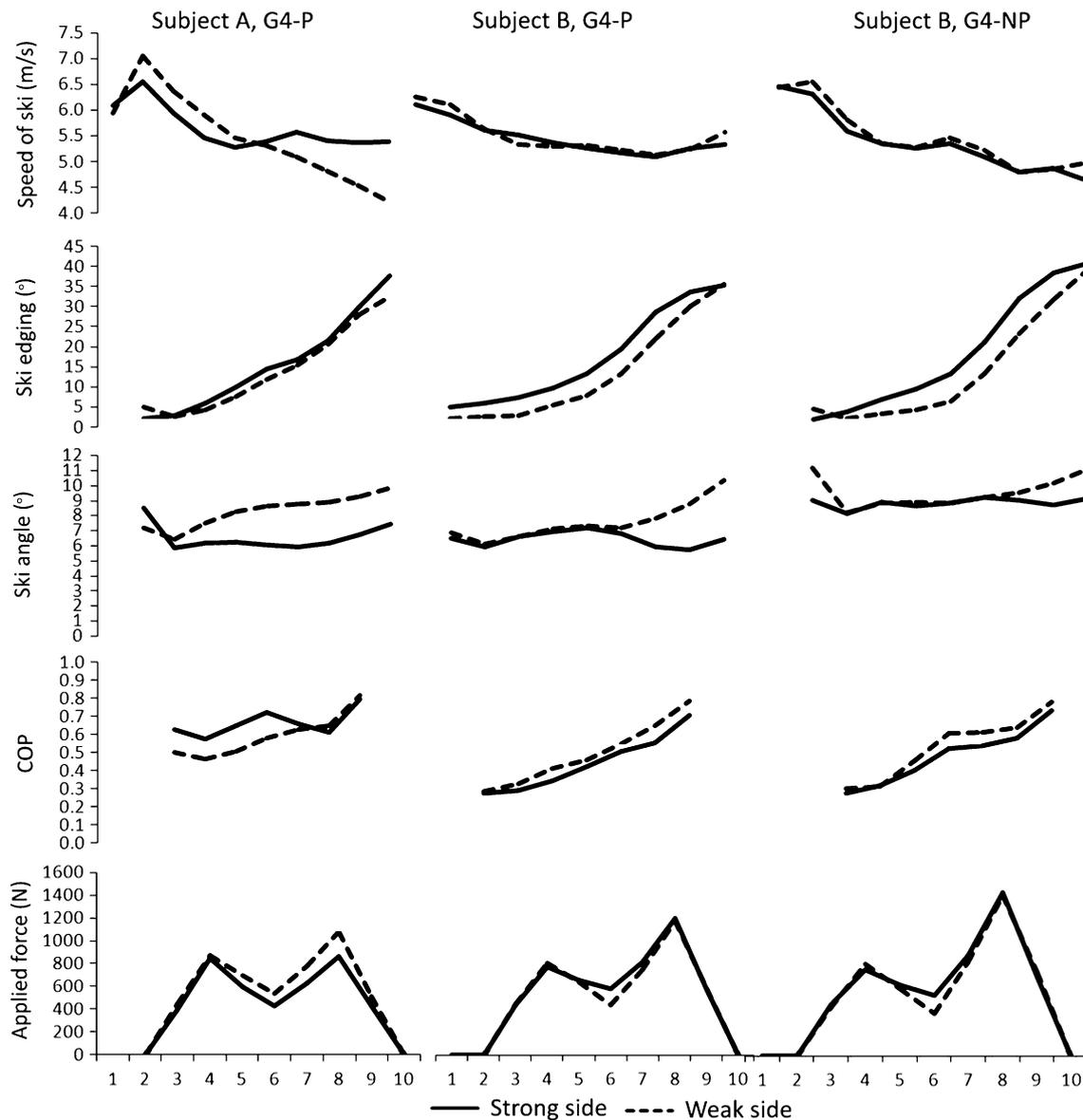
**Fig. 6** Comparisons of Skier A and B in the G4 skating technique (G4-P), as well as G4-P and G4 skating without poling (G4-NP) for Skier B during ten defined phases of the skating cycle. The skiing cycle are divided into ten segments according to Fig. 5. The applied force is the mean value of the measured forces during the ten cycles.
