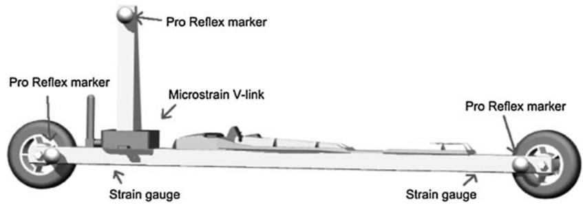
**Fig. 2** Definition of the calculated center of pressure and geometric values for calculating forces.  $L$  is the distance from the wheel to where the strain gauge is applied and  $h$  the height of the roller ski beam. The CoP found from the strain values in the front and back in the ski is recalculated into the fraction-value as shown in the figure, assuming a standard EU size 43 ski boot
