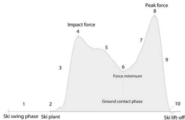
**Fig. 5** Definition of the different phases of a skating push-off. The force plot for one ski during a complete cycle divided in two phases; swing phase and ground contact phase. The peak force is defined as the largest force in the push off-phase (8). Force values, center of pressure, edging, angling and the speed of the skis are calculated for each of the distinct points 2, 4, 6, 8 and 10, as well as average values between these points; 1, 3, 5, 7 and 9
