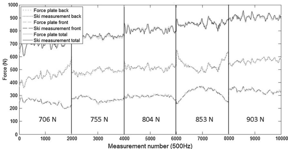
**Fig. 4** Comparisons of the roller ski and the force plate measurements, left ski. Five separate 4-s balance tests (the mass of subject with equipment is 72 kg) with ascending weights. The total applied
